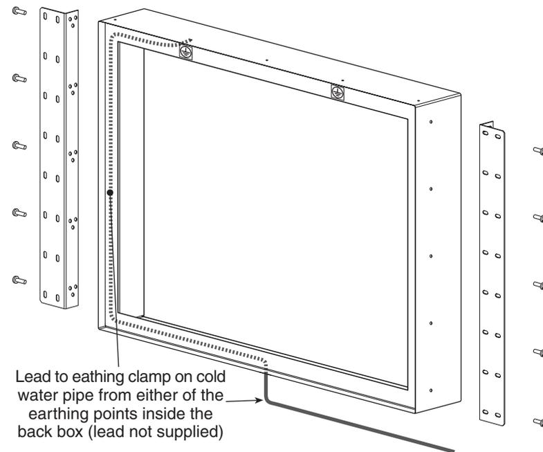
**Note:** Your qualified electrical installer must use one of the earthing strap screws as an earth point to earth the unit to ground.
