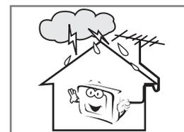
If an outside antenna is connected to the unit, ensure the external to internal cable entry is fully sealed
