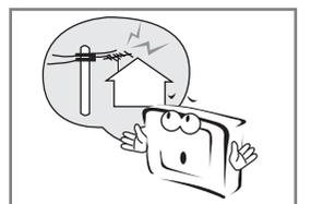
Ensure the antenna is located away from overhead cables.
