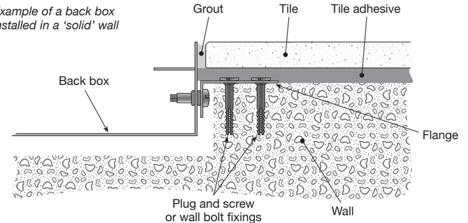
**Note:** Removal of the front glass requires a force of 100 lbs using a glass sucker, therefore, the box must be secured to the wall in such a manner to easily withstand such a pulling force.
