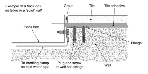
Note: Removal of the front glass requires a force of 100 lbs using a glass sucker, therefore, the box must be secured to the wall in such a manner to easily withstand such a pulling force.
