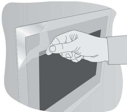
After the sealant has set the protective film can be removed from the front of the surround.
