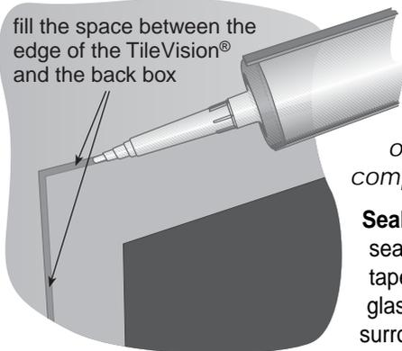
*This seal is essential for the reliable and safe operation of the TileVision® and must be completely waterproof.*
