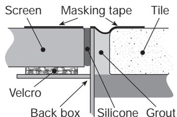
around the joint between the sides of the back box and TileVision®. Once the sealant has set and the masking tape removed the acrylic surround can be fitted as shown below.
