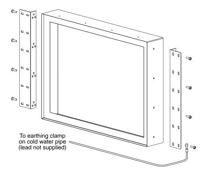
Note: Your qualified electrical installer must use one of the retaining screws as an earth point to earth the unit to ground.
