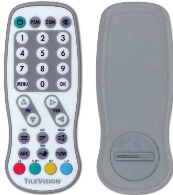
Waterproof remote control Grey case and battery cover Part number TVS/00208/04 Battery user replaceable with one CR2032 3V lithium button cell
