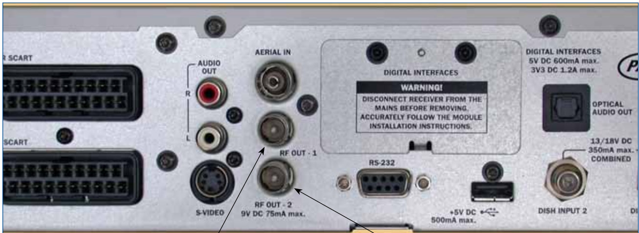
RF OUT - 1 – Main TV connection RF OUT - 2 – TileVision® connection
