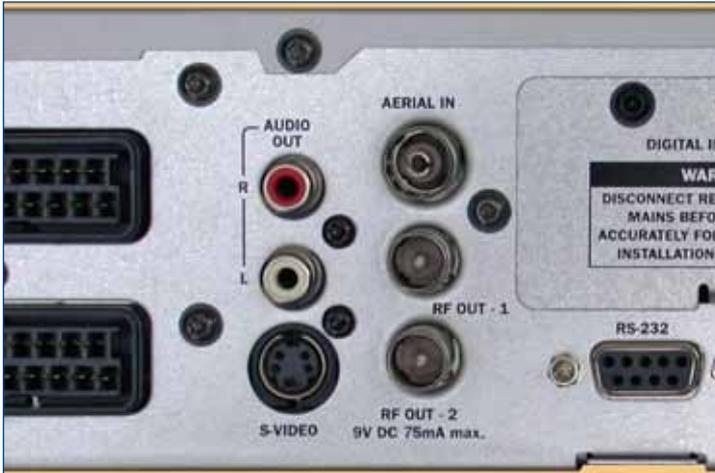
Note: The Remote Control Sender Unit (RCS Unit) is designed to work with Sky™ receivers that have 2 RF outputs. If the Sky™ receiver does not have 2 RF outputs, viewing the Sky™ channel (via the aerial connection) and remotely controlling the Sky™ receiver box from the TileVision® will not be possible.
