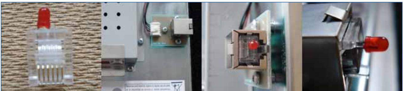
The TileVision® can be in either standby (red light on) or switched on (green light on). The light on the tester will light. Point the Sky™ remote control at the front of the TileVision®. On the Sky™ remote control, press a button (for example button 1) and keep it pressed, the light on the tester should flash. The light will flash very quickly. This concludes the test and demonstrates that the TileVision® will receive and send the remote control signals to the Sky™ receiver to control it.
